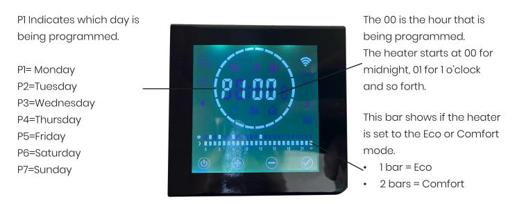
The + and - are used to set the either the comfort mode or reduced.
